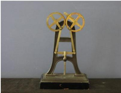
*Figure 15: Cartwright straight line mechanism*
