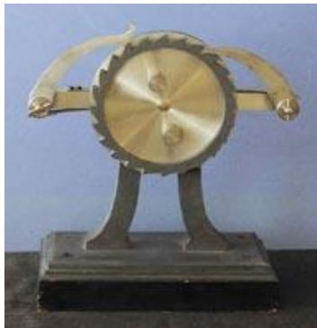
*Figure 16: Ratchet mechanism*
