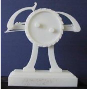
**Figure 17: 3-d printed copy of the ratchet mechanism**
