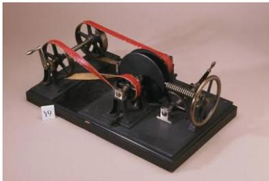
*Figure 13: Reversing belt transmission mechanism*
