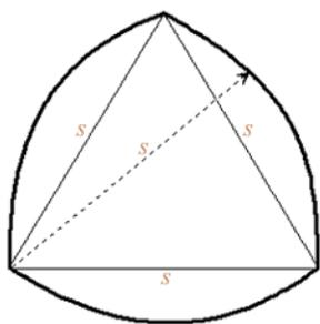
**Figure 4: Construction of Reuleaux triangle**
