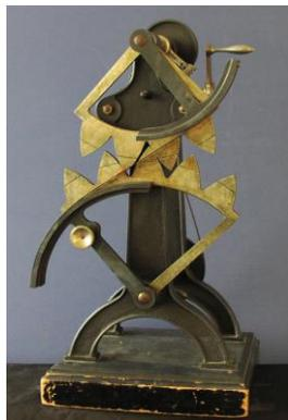
**Figure 7: Epicycloidal gear design**
