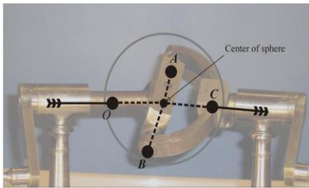
*Figure 12: Spherical geometry in the design of universal joint*
