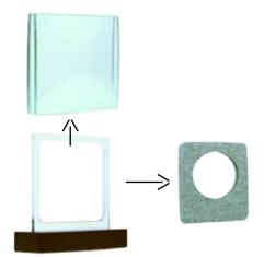
Lift the cap, push the felt inset out of the glass frame.
