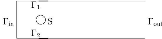
Let the goal of the simulation be the accurate computation of the effective force in the main flow direction imposed on the cylinder, i.e. the so-called ‘drag coefficient’,
