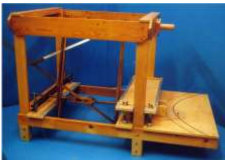
Figure 3: Instrument for hyperbolic lenses (Descartes)
