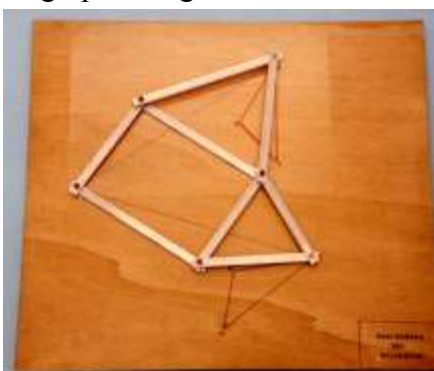
Figure 5: Pantograph of Sylvester (rotation)
